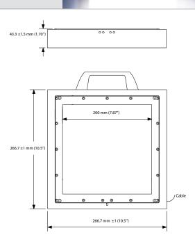
HSC Backlights by PHLOX®, designed for the Phantom®High Speed Camera offer the best luminance on the market
